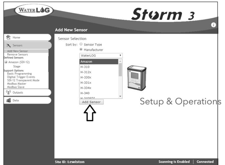
Figure 7: Add a new sensor by manufacturer
