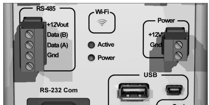
Figure 2: Storm3 Active and Power LED location
